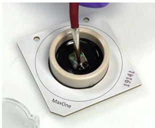
Figure 4. Position the organoid(s) onto the electrode array
